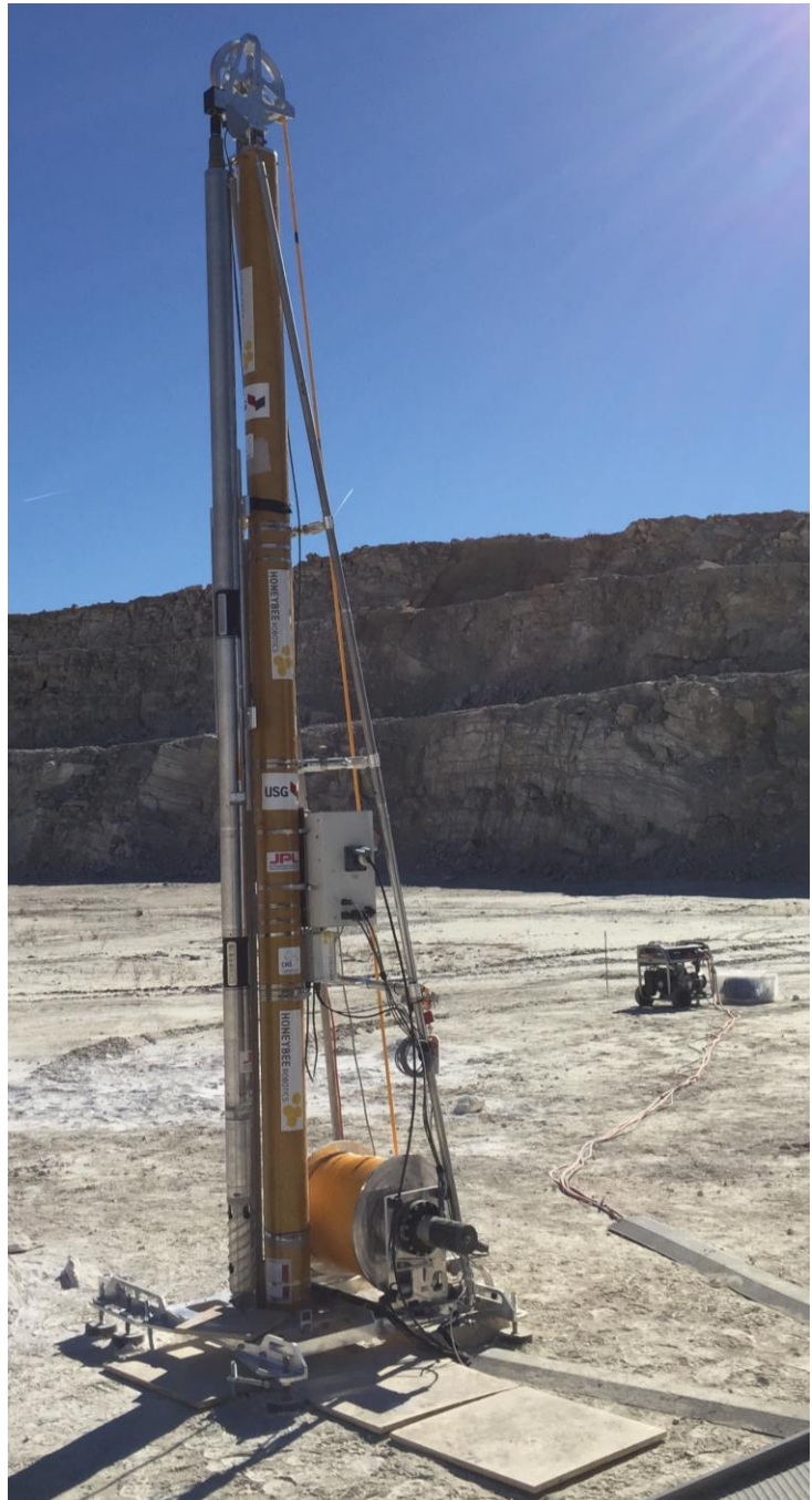
Figure 25: Auto-Gopher 2 deep drill during testing at the Fish Creek gypsum deposit in California (Davis, 2018). The drill and rig are both over 3 m tall. A generator can be seen in the background.
