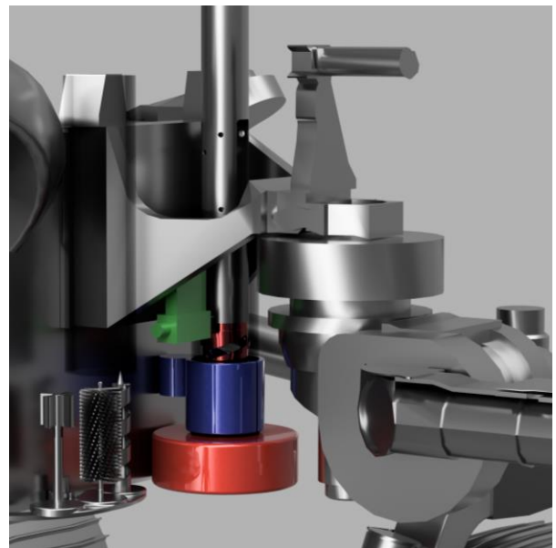
Figure 7: Assembly station mockup integrated into the mounting bracket for Perseverance's 5-DoF robot arm.
