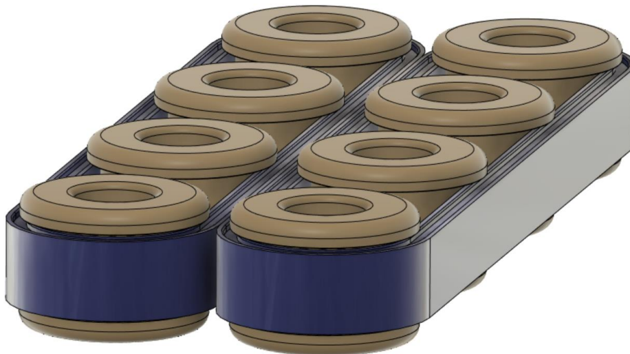
Figure 47 (above left): Cross-section view of the crowned pulley and thick belt option, designed to minimize crowding of the flange as recommended in Matthews, 2005.
