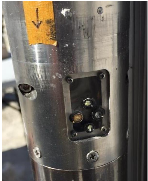
Figure 86: Optical / UV microscope integrated into Planetary Deep Drill (Zacny, 2016, Fig. 4).
