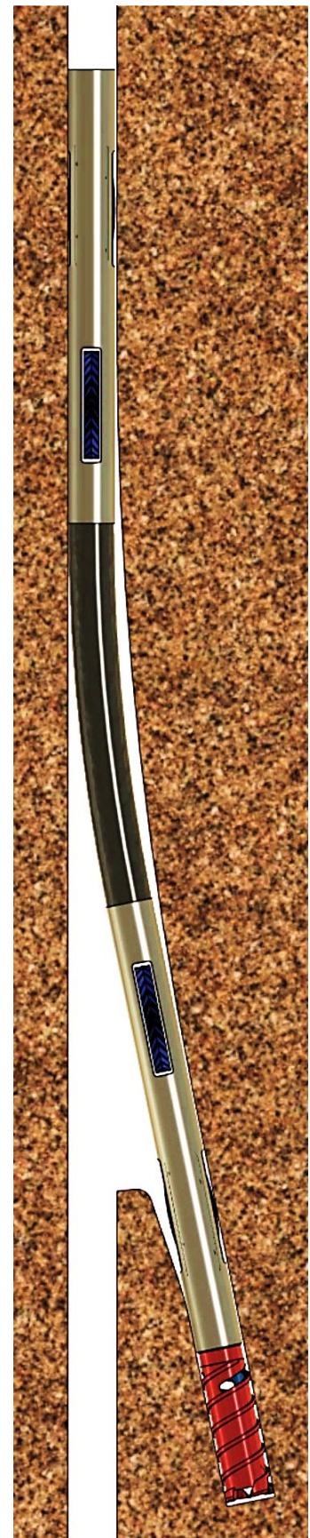
Figure 53: Branch bore drilling using an articulated joint.
