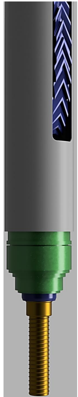
Figure 92 (above): Mockup of a re-sized chuck on a 64-mm borebot. Figure 93 (left): Hot needle ice core analysis tool. Shown is a standard medical-grade 7 gauge needle. Heating method TBD; likely an Inconel needle with a tapering thickness and an induction heater at the base of the needle.
